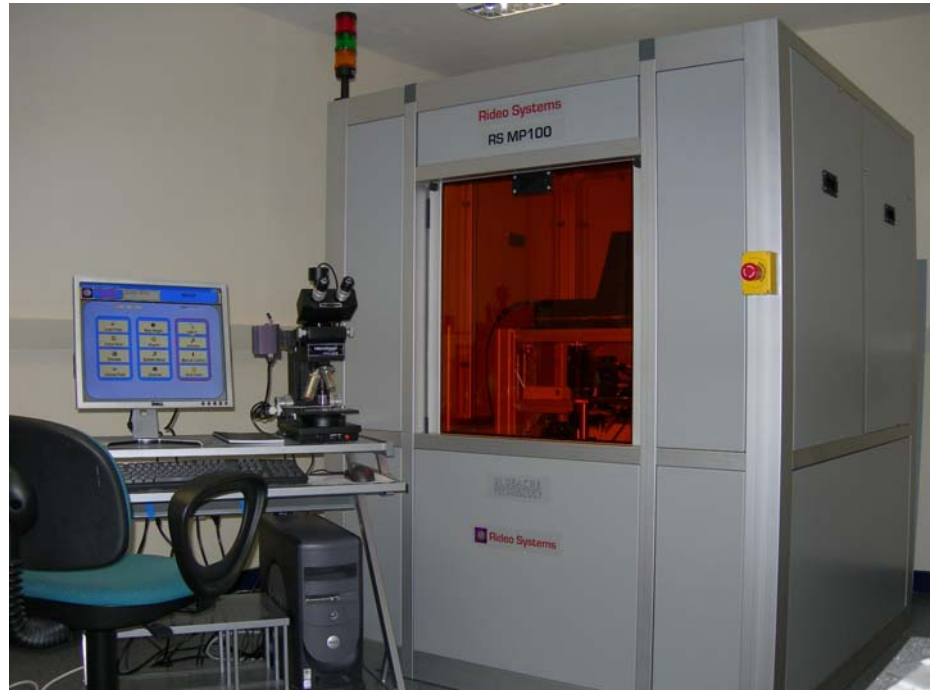
The RSMP100 micro machining platform fitted with a 355 nm Vanadate laser
